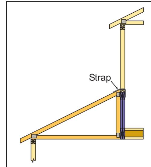
Figure 3. Wall girder protected from exterior exposure.
