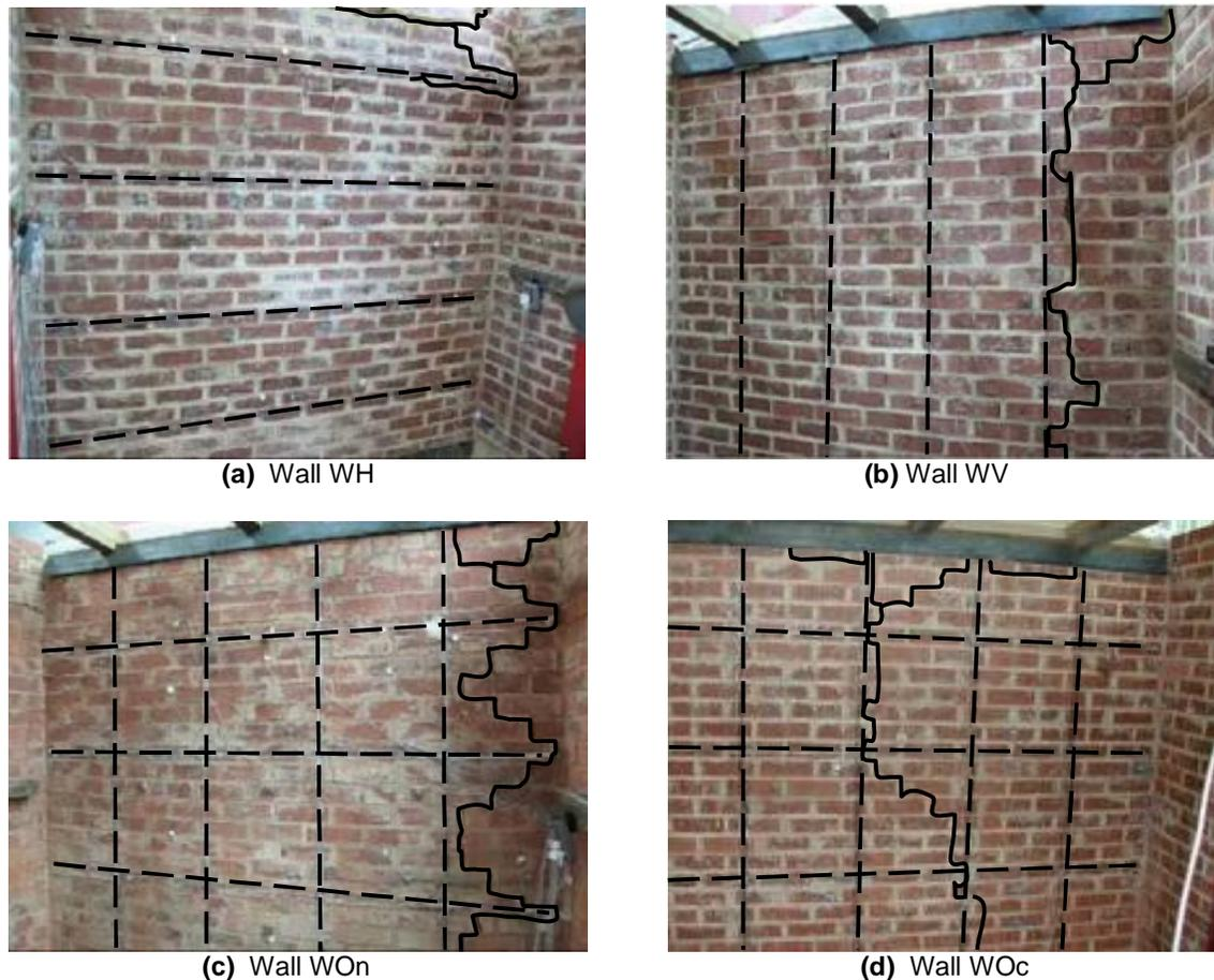
Fig. 4 Crack pattern of strengthened walls.
