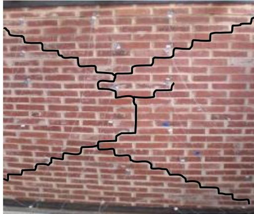
**Fig. 3** Crack pattern of wall WC.
